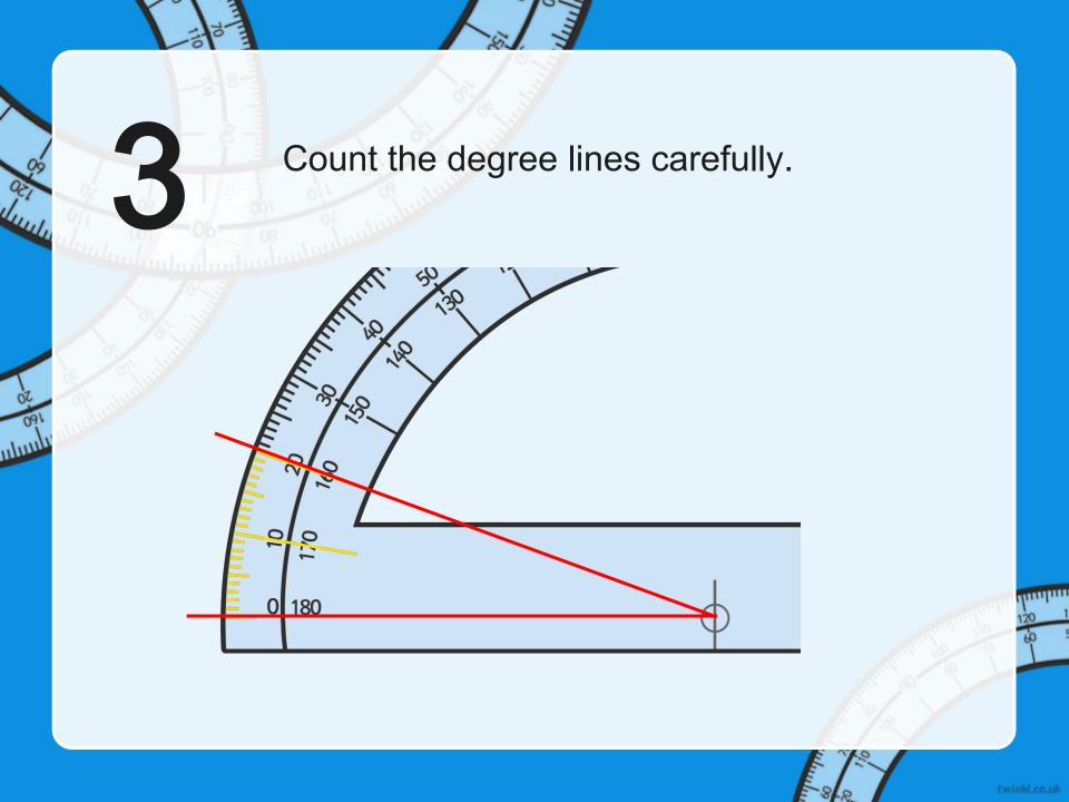
If the angle that you are measuring turns in an anti-clockwise direction, you will need to use the inner scale of your protractor.
