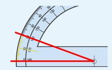
Use the inner scale of your protractor if the angle turns in an anti-clockwise direction..
